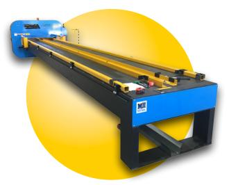
The BeautPress Xpress is an Australian built, platen style floor truss press. It is available in both a 600mm wide version for building single floor trusses and a 1200mm version for building two floor trusses simultaneously.
