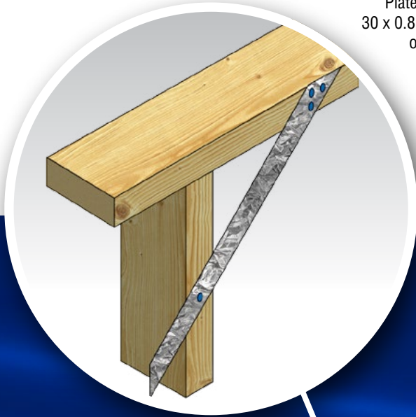
SpeedBrace fixed with 1 MiTek nail to each stud and 3 MiTek nails to each wall plate.
